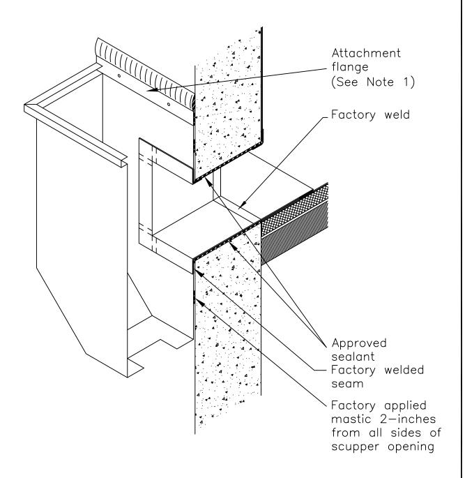
Note 1: Back seal and fasten top flange of collector 6—inches on center. Apply a bead of approved sealant on top of flange.
