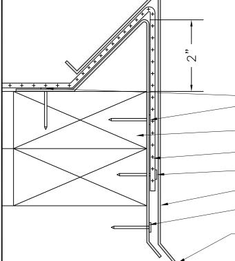
Fasten waterdam in pre—punched—holes 12" o.c. using 1—1/4" Galv.—ring shank roofing nails or #14 screw
